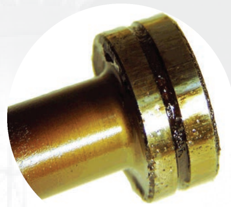
IGV valves and fuel control valves are typically the first problem components
