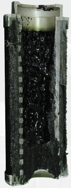
Filter element cross section ( Lacquer Varnish Deposits, Support Tube )
